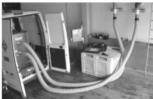
Fig. 7 The HDS 800 in a fumigation van with a two-hose connection to a fruit fumigation chamber.
